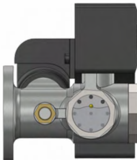
Good Level, Does Not Need Oil
